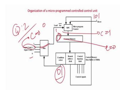
So, here I have a connected carry 0. So, if I put the 01 say then this line will be 1 if and only if carry bit equal to 1, and this line is going to be a 0 if the carry bit equal to 0 so that means what, if I put selection condition as 01 and if the carry bit is a 1 so you are going to load 101. I put a
