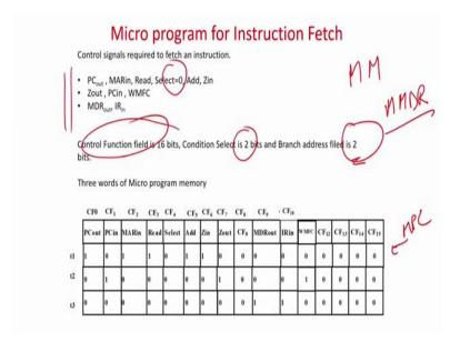
This memory location will be read from the micro-program memory it will go to the micro-program memory data register, and this one this point actually will be connected to the program counter in, this memory data bus micro-program memory data bus will be connected to the *PC* input, this will be connected to the *MAR* input, this will be connected to the read port of the main memory and so, forth.
