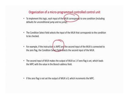
So, basically whatever I have told you is actually written in the slide. So, to implement this logic we actually this use a multiplexer. So, the multiplexer corresponds to jump unconditional, jump conditional and just increment basically the, that is what is the case. So, if it is a jump on 0. So, some 0 flag has to be checked.
