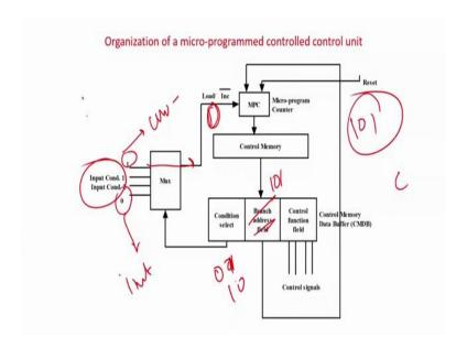
So, I will put the condition as 00 which is the default condition in which it's a jump unconditional. So, if I put 00 the first bit of the multiplexer will be connected to the output, and here I have put a default 1. So, in that case this line is always going to 1 and you are by default jump to 101, which is specified over here. So, this is how actually it is implemented.
